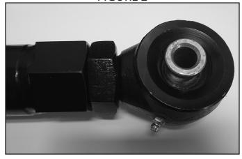
8. Attach the Traction Bar to the axle bracket with a 9/16" x 4" bolt, 9/16" nut and 9/16" SAE washers from Bolt Pack 964. Install the traction bar so that the Forged Flex End (A171) is mounted to the axle bracket. Leave mounting hardware loose at this time
